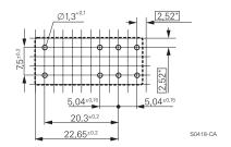
\*) With the recommended PCB hole sizes a grid pattern from 2.5mm to 2.54mm can be used.
