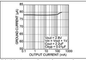
FIGURE 2-3: Ground Current vs. Output Current.
