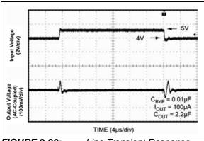
**FIGURE 2-20:** Line Transient Response (3.0V Fixed Output Version).
