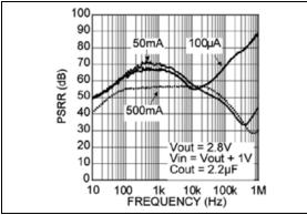
**FIGURE 2-1:** PSRR (Bypass Pin Capacitor =  $0.1 \mu$ F).
