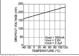
FIGURE 2-14: Dropout Voltage vs. Temperature.
