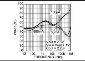
FIGURE 2-2: PSRR (Bypass Pin Capacitor =  $0.01 \mu$ F).
