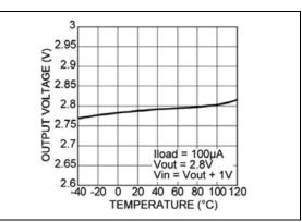
FIGURE 2-17: Output Voltage vs. Temperature.
