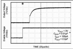
FIGURE 2-22: Enable Pin Delay (3.0V Fixed Output Version).
