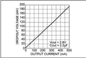
FIGURE 2-15: Dropout Voltage vs. Load Current.
