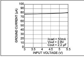
FIGURE 2-8: Ground Current vs. Input Voltage.
