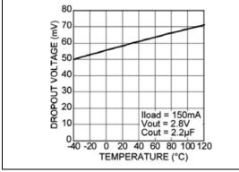
FIGURE 2-13:Dropout Voltage vs.Temperature.
