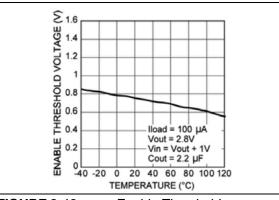
FIGURE 2-18:Enable Threshold vs.Temperature.
