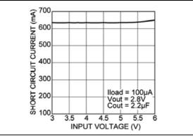
FIGURE 2-16: Short-Circuit Current vs. Input Voltage.
