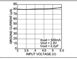
FIGURE 2-10: Ground Current vs. Input Voltage.
