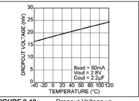
FIGURE 2-12:Dropout Voltage vs.Temperature.
