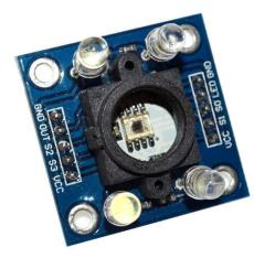
Description: Chip: TCS3200 Input voltage: DC 3 ~ 5V Output frequency voltage: 0 ~ 5V Use bright white LED lights Can be connected directly with Microcontroller Static detection of the measured object color Best detection distance: 10mm
