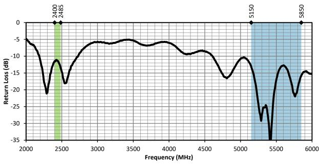
Figure 11. LPD Return Loss, Straight, with Frequency Band Highlights
