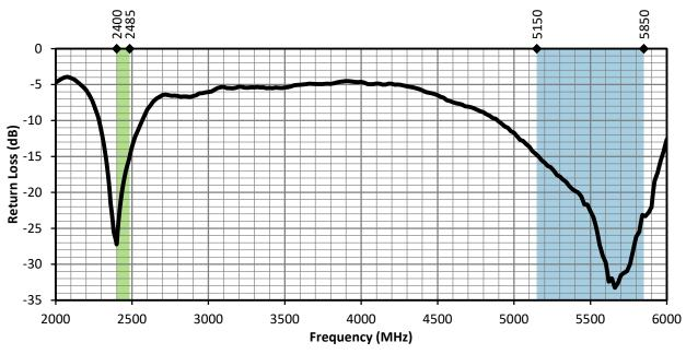
Figure 4. LPD Return Loss, Bent-90, with Frequency Band Highlights
