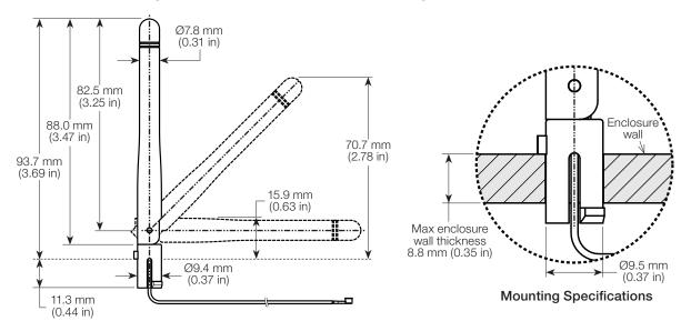
Figure 1. ANT-DB1-LPD-125 Dimensions and Mounting Data
