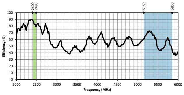
Figure 7. LPD Radiation Efficiency, Bent-90, with Frequency Band Highlights
