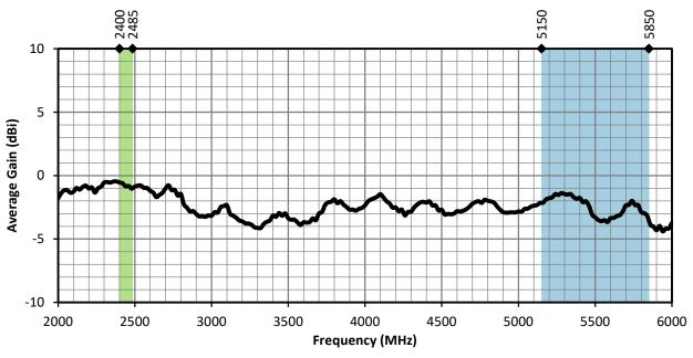
Figure 6. LPD Average Gain, Bent-90, with Frequency Band Highlights
