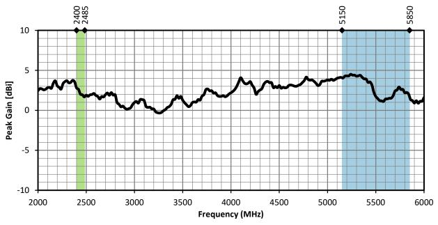
Figure 5. LPD Peak Gain, Bent-90, with Frequency Band Highlights
