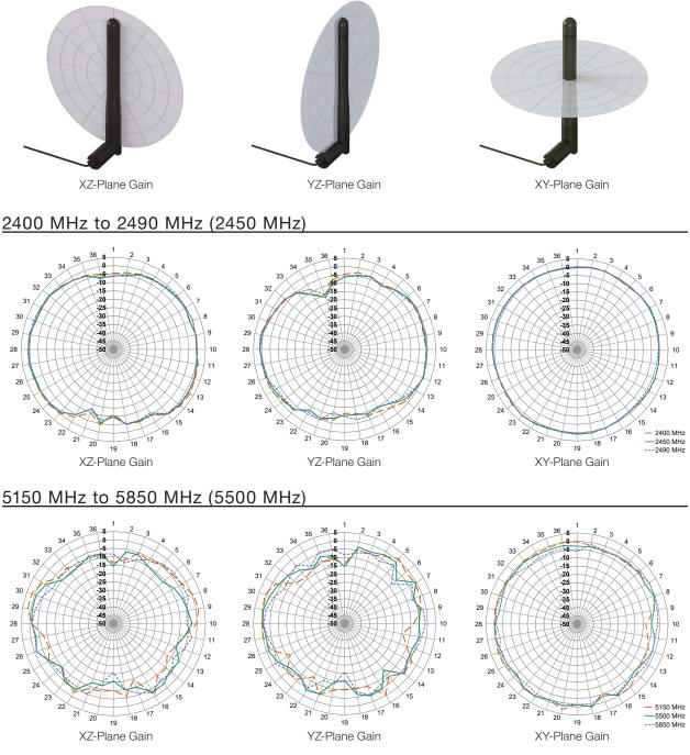
Figure 8. Radiation Patterns for LPD, Bent-90
