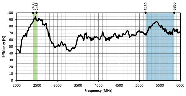
Figure 14. LPD Radiation Efficiency, Straight, with Frequency Band Highlights
