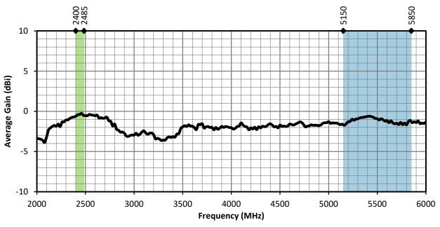
Figure 13. LPD Average Gain, Straight, with Frequency Band Highlights
