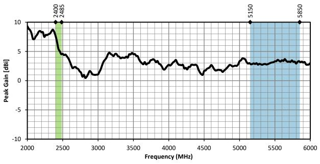
Figure 12. LPD Peak Gain, Straight, with Frequency Band Highlights
