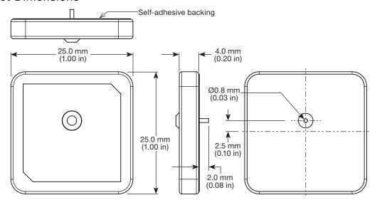
Figure 1. 868-CPA Antenna Dimensions
