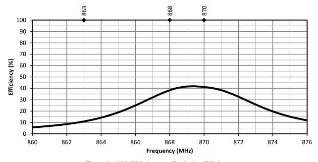
Figure 5. 868-CPA Antenna Radiation Efficiency
