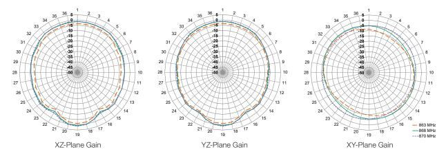
Figure 6. Radiation Patterns for 868-CPA Antenna
