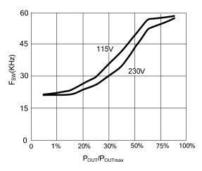
Fig.1 The relation curve between f<sub>SW</sub> and relative output power P<sub>OUT</sub>/ P<sub>OUT (MAX)</sub>
