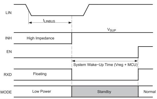
Figure 5. Wake-Up Via LIN Bus Timing Diagram
