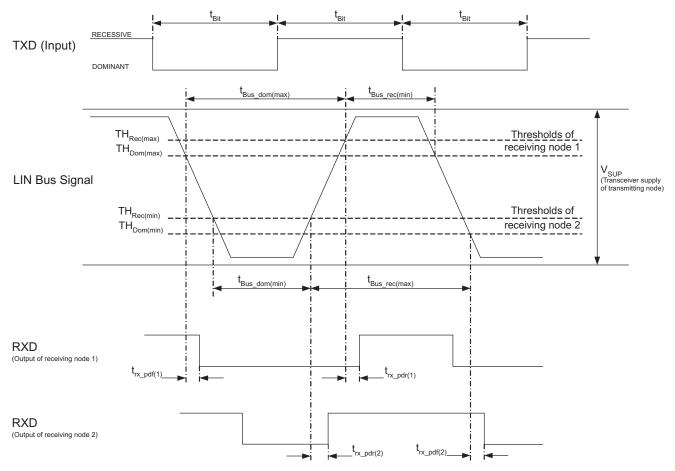
Figure 1. Definition of Bus Timing Parameters
