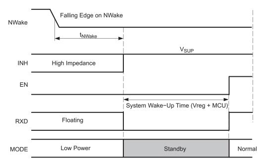
Figure 6. Wake-Up Via NWake Timing Diagram
