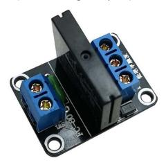
1. 5V Omron solid state relays 250V 2A, output with resistive Insurance Wire 250V 2A.
