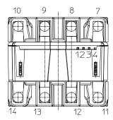
The four integrated primary conductors have a diameter of 4.5 mm.
