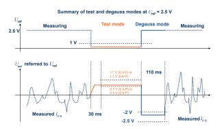
The activation of degauss takes typically 40  $\mu$ s after releasing  $U_{ref}$  pin, then degauss lasts typically 110 ms.
