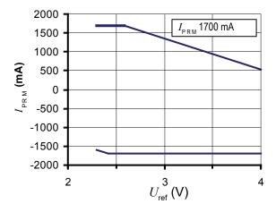
$\begin{array}{ll} \mbox{Upper limit: } I_{\rm p} = 1700 \mbox{ mA} & (U_{\rm ref} = 2.3 \hdots 2.625 \mbox{ V}) \\ \mbox{Upper limit: } I_{\rm p} = -833.3 \ ^* U_{\rm ref} + 3854.2 & (U_{\rm ref} = 2.625 \hdots 2.4 \mbox{ V}) \\ \mbox{Lower limit: } I_{\rm p} = -833.3 \ ^* U_{\rm ref} + 312.5 & (U_{\rm ref} = 2.3 \hdots 2.375 \mbox{ V}) \\ \mbox{Lower limit: } I_{\rm p} = -1700 \mbox{ mA} & (U_{\rm ref} = 2.375 \hdots 2.375 \hdots 4 \mbox{ V}) \\ \end{array}$
