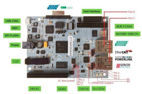
Figure 3. AM3359 ICE 2.1 EVM Connector and Jumper Loactions
