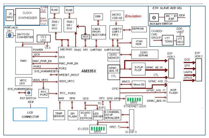
Figure 4. AM335x ICE Rev. 2.1 EVM Block Diagram
