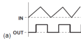
Figure 7. Schmitt Trigger Curves
