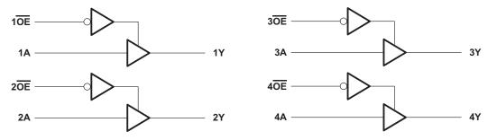
Figure 4. Logic Diagram (Positive Logic)
