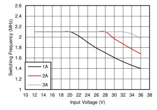
Figure 19. Switching Frequency versus Input Voltage  $V_{\rm OUT}$  = 3.3 V
