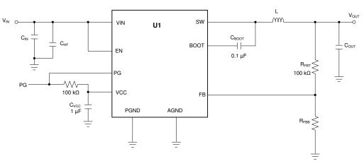
Figure 50. Circuit for Application Curves
