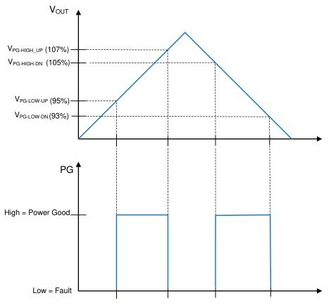
Figure 7. Static Power-Good Operation
