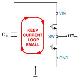
Figure 51. Current Loops with Fast Edges
