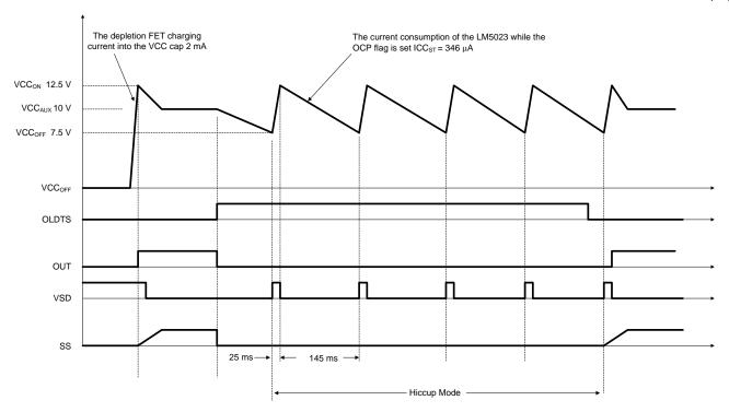
Figure 17. Hiccup Mode Timing
