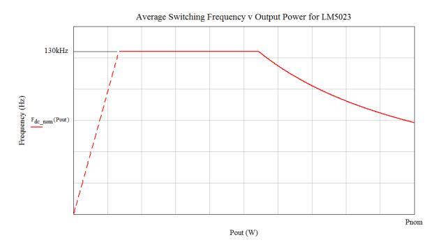
Figure 13. LM5023 Modulation Curve
