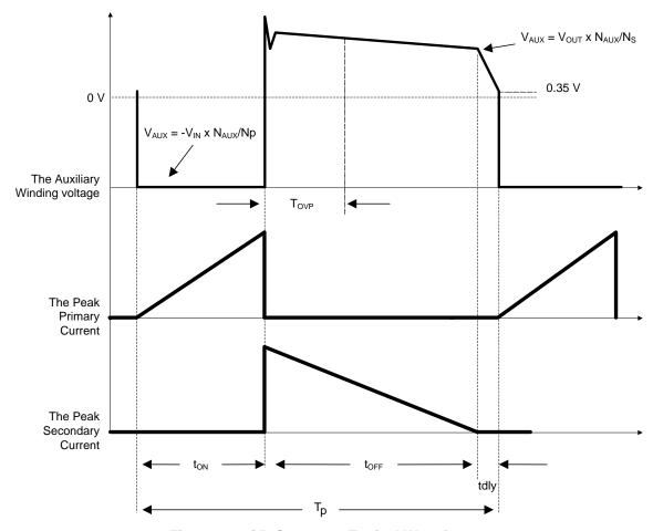
Figure 12. QR Converter Typical Waveforms
