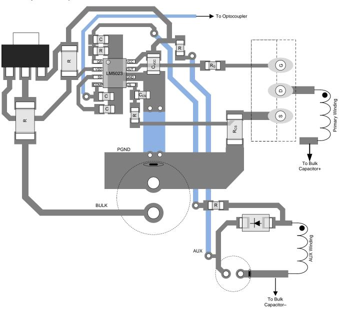
Figure 25. LM5023 Layout Example
