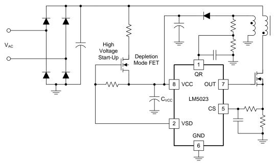
Figure 9. Start-Up With a Depletion Mode FET
