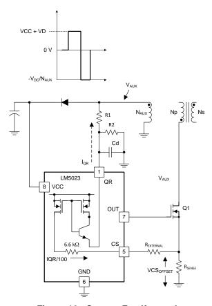
Figure 16. Current Feedforward
