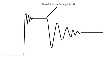
Figure 11. The Flyback Drain Voltage Waveform
