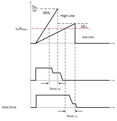
Figure 15. Line-Current Feedforward
