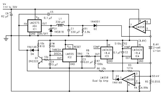
Figure 20. (Fast) Pulsed Constant Current 2-Cell Charger
