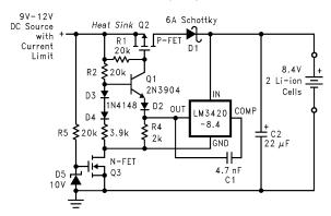
Figure 21. MOSFET Low Dropout Charger
