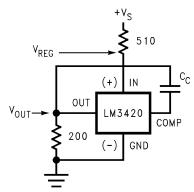
Figure 8. Circuit Used For Bode Plots
