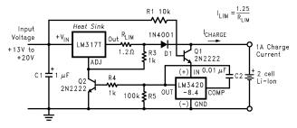
Figure 14. Constant Current/Constant Voltage Li-Ion Battery Charger
