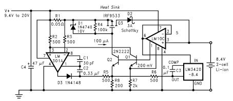
Figure 16. Low Dropout Constant Current/Constant Voltage 2-Cell Charger
