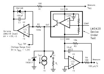
Figure 10. LM3420 Test Circuit
