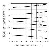
Figure 11. Normalized Temperature Drift With Output Externally Trimmed
