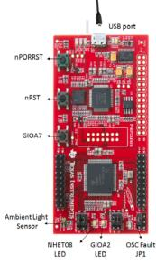
Upon detecting the fault, on-board Hercules MCU will respond by asserting the error pin (nERROR) low, indicated by the red LED on the bottom right corner of the board. **Note:** Open jumper JP1 and reset the board before continuing with other demos.
