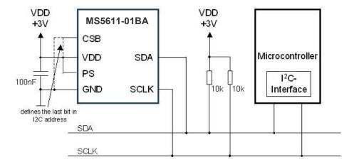
Figure 17: Typical application circuit with SPI / I<sup>2</sup>C protocol communication
