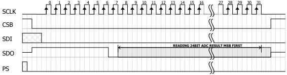
Figure 8: ADC Read sequence
