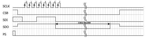
Figure 5: Reset command sequence SPI mode 0
