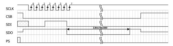
Figure 6: Reset command sequence SPI mode 3
