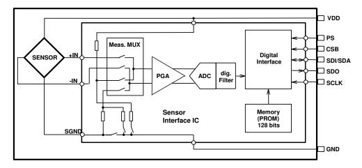
Figure 1: Block diagram of MS5611-01BA
