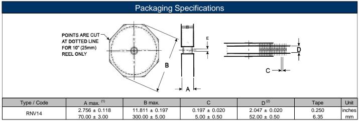
Dimension "E": This is a non-critical dimension that does not have a tolerance in the standard. Range of diameters is from 0.547" (13.9 mm) to 1.5" (38.1 mm)
