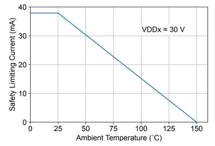
Figure 4.6. DFN-14 Thermal Derating Curve, Dependence of Safety Limiting Values per VDE
