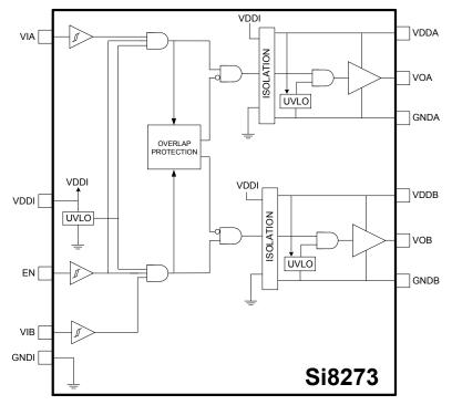
Figure 2.2. Si8273 Block Diagram
