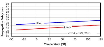
Figure 2.14. Propagation Delay vs. Temperature
