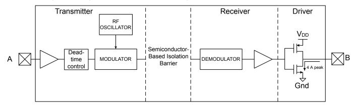
Figure 2.5. Simplified Channel Diagram
