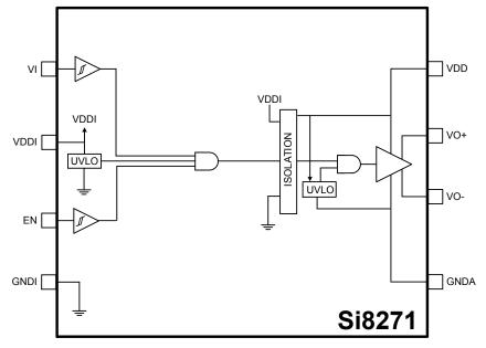
Figure 2.1. Si8271 Block Diagram
