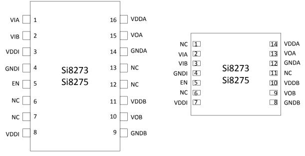
Figure 5.2. Pin Assignments Si8273/5
