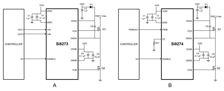
Figure 3.1. Si827x in Half-Bridge Application
