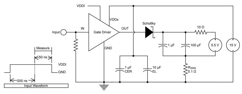
Figure 4.2. IOH Source Current Test Circuit
