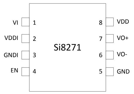
Figure 5.1. Pin Assignments Si8271
