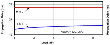
Figure 2.13. Propagation Delay vs. Load
