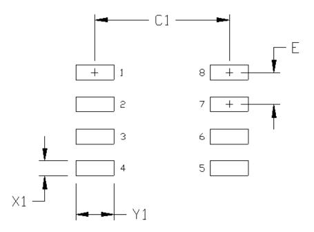
Figure 7.2. 8-Pin Narrow Body SOIC Land Pattern
