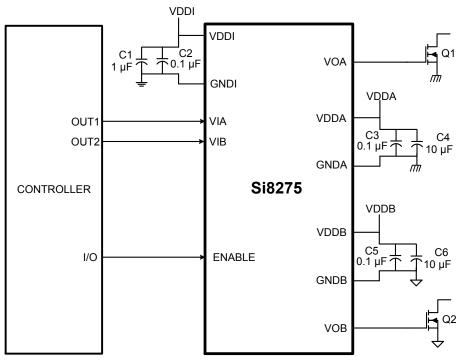
Figure 3.2. Si827x in a Dual Driver Application
