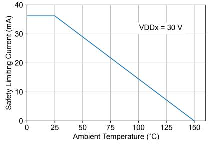
Figure 4.4. NB SOIC-8 Thermal Derating Curve, Dependence of Safety Limiting Values per VDE
