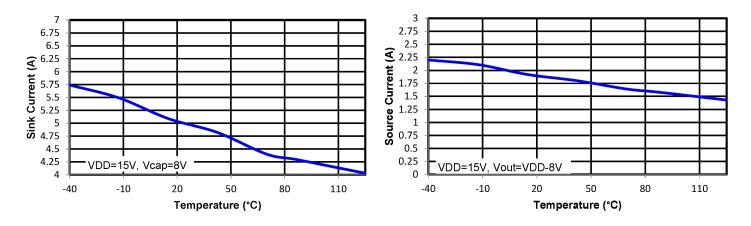
Figure 2.15. Output Sink Current vs. Temperature
