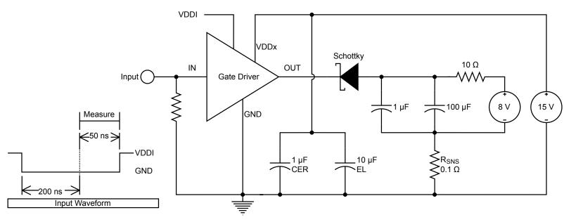
Figure 4.1. IOL Sink Current Test Circuit
