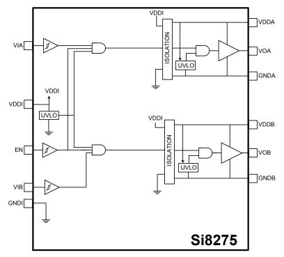
Figure 2.4. Si8275 Block Diagram
