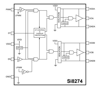
Figure 2.3. Si8274 Block Diagram
