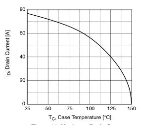
Figure 10. Maximum Drain Current vs. Case Temperature
