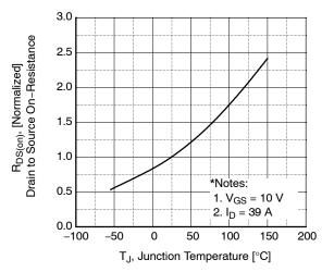
Figure 8. On-Resistance Variation vs. Temperature
