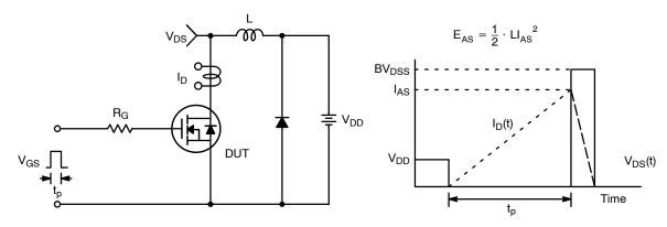
Figure 15. Unclamped Inductive Switching Test Circuit & Waveforms
