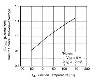
Figure 7. Breakdown Voltage Variation vs. Temperature
