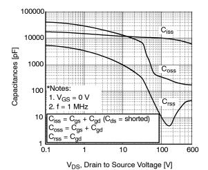
Figure 5. Capacitance Characteristics
