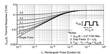
Figure 12. Transient Thermal Response Curve
