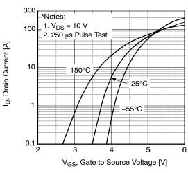
Figure 2. Transfer Characteristics
