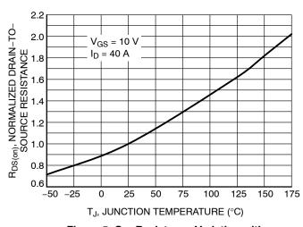
Figure 5. On–Resistance Variation with Temperature
