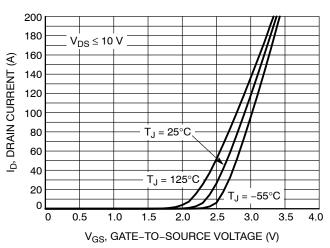
Figure 2. Transfer Characteristics
