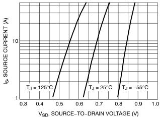
Figure 10. Diode Forward Voltage vs. Current
