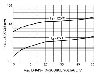
Figure 6. Drain-to-Source Leakage Current vs. Voltage
