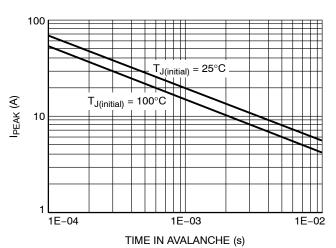
Figure 12. I<sub>PEAK</sub> vs. Time in Avalanche
