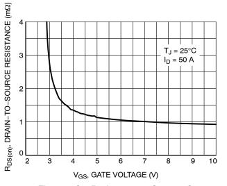
Figure 3. On-Resistance vs. Gate-to-Source Voltage
