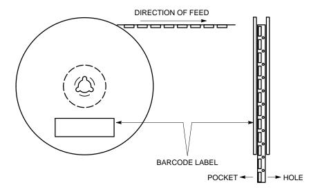
Figure 8. Reel Winding Direction
