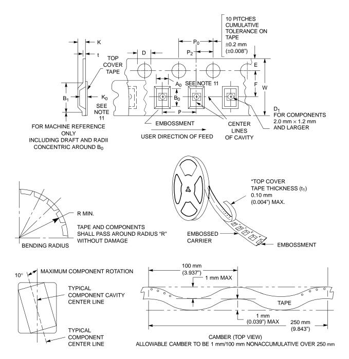
11. A<sub>0</sub>, B<sub>0</sub>, and K<sub>0</sub> are determined by component size. The clearance between the components and the cavity must be within 0.05 mm min to 0.50 mm max. The component cannot rotate more than 10° within the determined cavity
