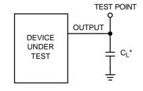
\*Includes all probe and jig capacitance Figure 4. Test Circuit
