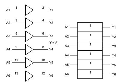
Figure 1. Logic Diagram
