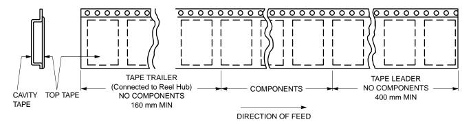
Figure 9. Tape Ends for Finished Goods
