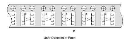
Figure 10. TSSOP and SOIC R2 Reel Configuration/Orientation
