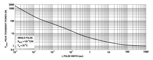
Figure 13. Single Pulse Maximum Power Dissipation
