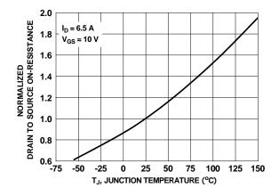
Figure 3. Normalized On-Resistance vs. Junction Temperature
