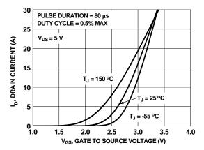
Figure 5. Transfer Characteristics
