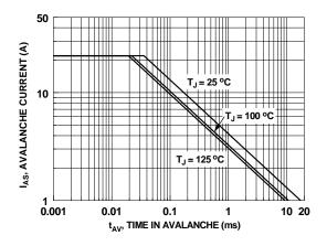
Figure 9. Unclamped Inductive Switching Capability
