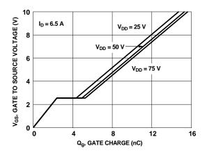
Figure 7. Gate Charge Characteristics
