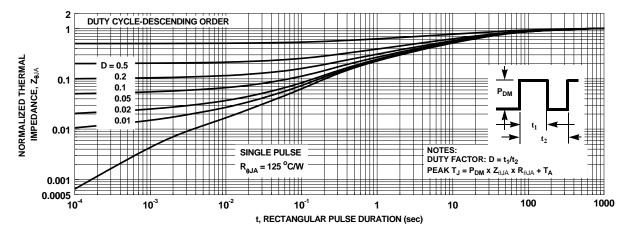
Figure 14. Junction-to-Ambient Transient Thermal Response Curve
