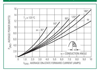
Figure 3. On-State Characteristics
