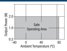
UL60950 recognition to a maximum ambient temperature of 85°C and/or case temperature limit of 155°C, measured on the face opposite the pins.
