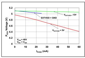
**FIGURE 2-9:**  $P_{VDD}$  Load Regulation.
