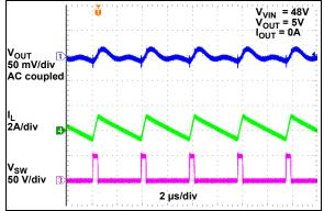
**FIGURE 2-55:** Switching Waveform at No Load (CCM Mode).
