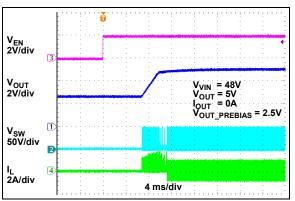
FIGURE 2-40: Enable Turn-On with Prebiased Output (CCM Mode).
