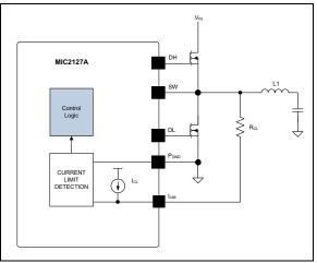
FIGURE 4-4: MIC2127A Current Limiting Circuit.
