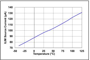
**FIGURE 2-16:** I<sub>LIM</sub> Source Current vs. Temperature.
