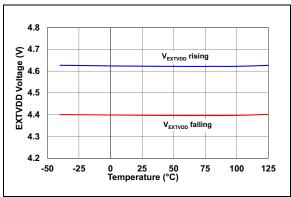
**FIGURE 2-11:** EXTVDD Threshold vs. Temperature.
