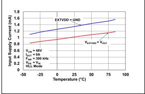
**FIGURE 2-4:** Input Supply Current vs. Temperature (HLL Mode).
