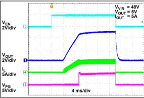
FIGURE 2-35: Enable Turn-On/Turn-Off.
