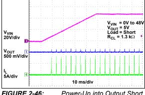
FIGURE 2-46: Power-Up into Output Short.
