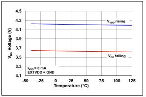
**FIGURE 2-10:**  $V_{DD}$  UVLO Threshold vs. Temperature.
