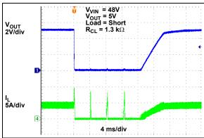
FIGURE 2-49: Recovery from Output Short Circuit.
