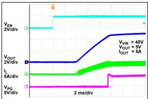
FIGURE 2-36: Enable Turn-On Delay.
