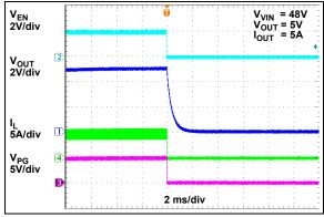
FIGURE 2-37: Enable Turn-Off Delay.
