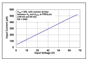
FIGURE 2-5: Input Shutdown Current vs. Input Voltage.
