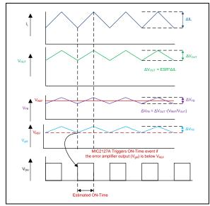
**FIGURE 4-1:** MIC2127A Control Loop Timing.
