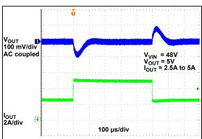
FIGURE 2-54: Load Transient Response (HLL Mode).
