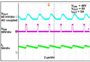
**FIGURE 2-57:** Switching Waveform at Full Load.
