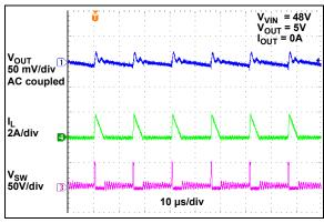
**FIGURE 2-56:** Switching Waveform at No Load (HLL Mode).
