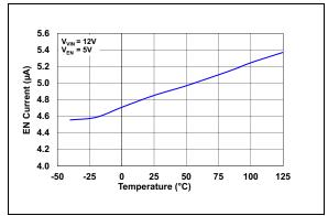
**FIGURE 2-13:** Enable Bias Current vs. Temperature.
