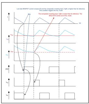
FIGURE 4-3: MIC2127A Control Loop Timing (HLL Mode).
