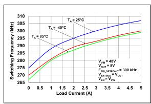
**FIGURE 2-15:** Switching Frequency vs. Load Current.
