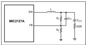
FIGURE 5-5: Inadequate Ripple at FB.
