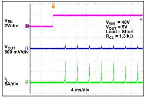
**FIGURE 2-45:** Enable into Output Short.
