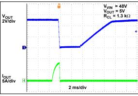
FIGURE 2-47: **Output Current Limit** Threshold.
