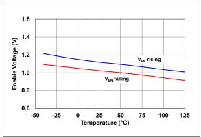
**FIGURE 2-12:** Enable Threshold vs. Temperature.
