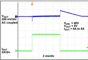
FIGURE 2-51: Load Transient Response (HLL Mode).
