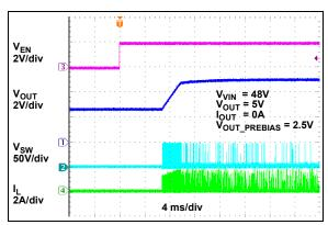
FIGURE 2-41: Enable Turn-On with Prebiased Output (HLL Mode).
