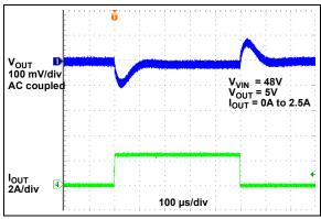
FIGURE 2-52: Load Transient Response (CCM Mode).
