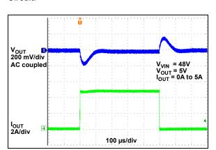
FIGURE 2-50: Load Transient Response (CCM Mode).
