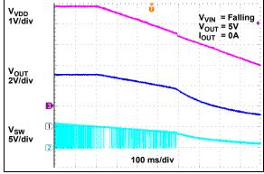
FIGURE 2-44: V<sub>DD</sub> UVLO Threshold-Falling.
