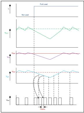
**FIGURE 4-2:** MIC2127A Load Transient Response.
