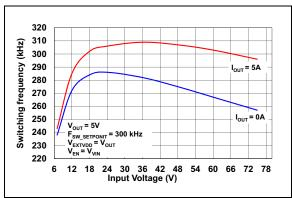
**FIGURE 2-14:** Switching Frequency vs. Input Voltage.
