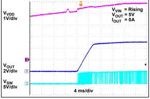
**FIGURE 2-43:** V<sub>DD</sub> UVLO Threshold-Rising.
