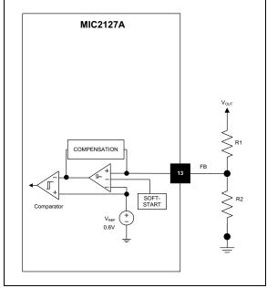
FIGURE 5-3: Output Voltage Adjustment.
