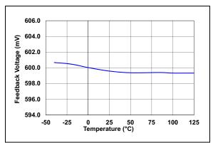
**FIGURE 2-18:** Feedback Voltage vs. Temperature.
