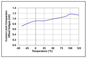
**FIGURE 2-17:** Current Limit Comparator Offset vs Temperature.
