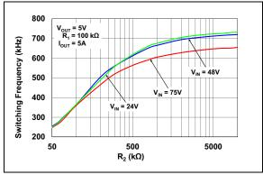
FIGURE 5-2: Switching Frequency vs. R<sub>2</sub>.
