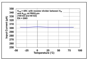
**FIGURE 2-6:** Input Shutdown Current vs. Temperature.
