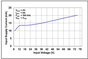
**FIGURE 2-1:** Input Supply Current vs. Input Voltage.
