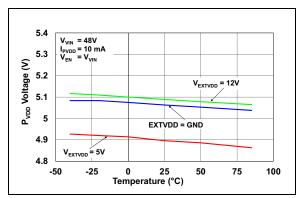
**FIGURE 2-8:** P<sub>VDD</sub> Voltage vs. Temperature.
