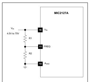
FIGURE 5-1: Switching Frequency Adjustment.
