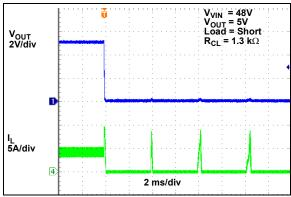
**FIGURE 2-48:** Output Short Circuit.
