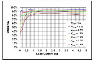
FIGURE 2-25: Efficiency vs. Output Current (Input Voltage = 12V, HLL Mode).
