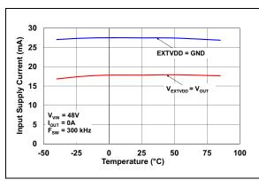
**FIGURE 2-2:** Input Supply Current vs. Temperature.
