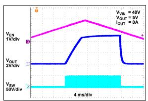
FIGURE 2-42: Enable Thresholds.
