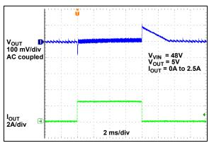
FIGURE 2-53: Load Transient Response (HLL Mode).
