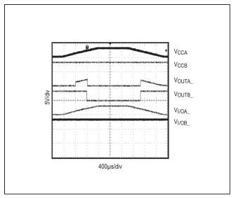
Figure 3. Undervoltage Lockout Behavior
