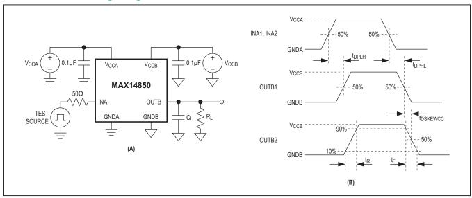
Figure 1. Test Circuit (A) and Timing Diagram (B) for Unidirectional Channels
