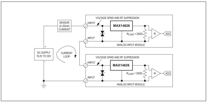
Figure 1. 4–20mA Current Loop Sensor Application
