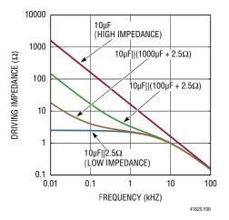
Figure 9. Aggregate Input Impedance vs Frequency
