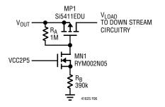
Figure 6. Isolating Downstream Circuits in Ship Mode.
