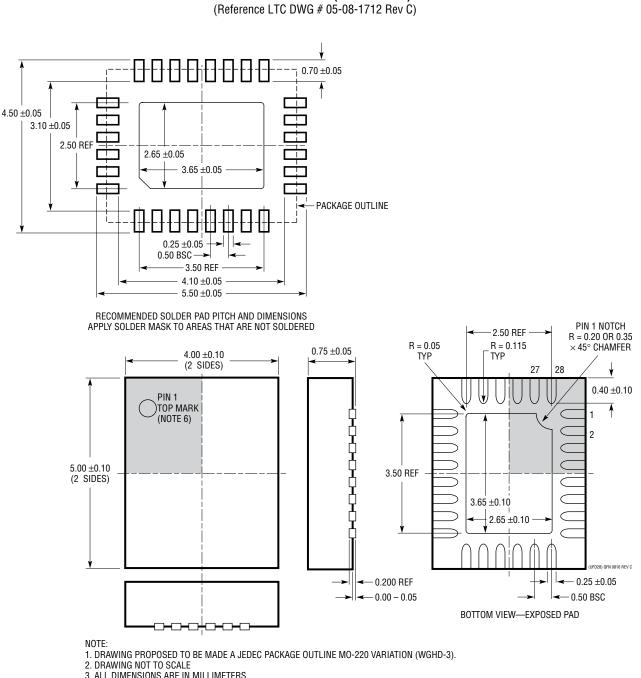
**UFD Package** 28-Lead Plastic QFN ( $4mm \times 5mm$ )
