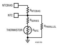
Figure 3. Diluting the Thermistor with Low Drift Series and Parallel Resistors
