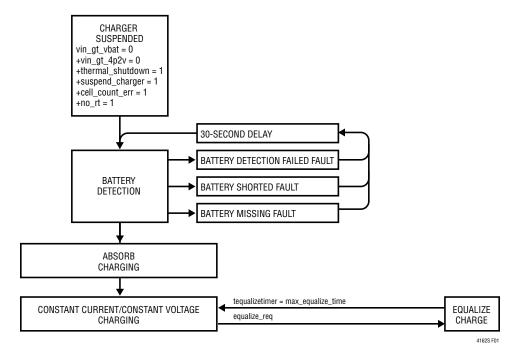
Figure 1. Battery Charging State Diagram
