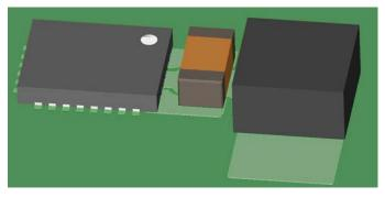
Figure 13. Recommended Placement of the V<sub>OUT</sub> Bypass Capacitor and Inductor
