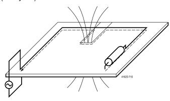
Figure 10. Currents Tend to Follow Their Natural Least Area Path. Breaks in the Ground Plane Lead to Increased Impedance and EMI
