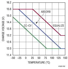
Figure 2. 12V Lead-Acid Temperature Profile
