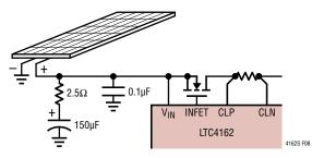
Figure 8. Input Impedance Compensation Network
