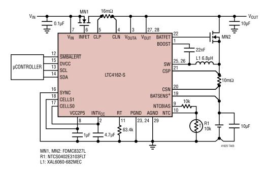
32V to 24V 3.2A Charger with PowerPath and 2A Input Limit
