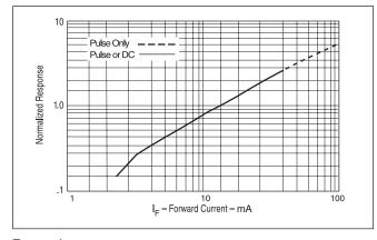
FIGURE 1. Normalized power launched versus forward current
