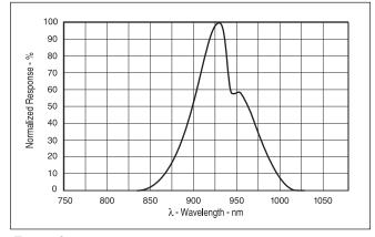
FIGURE 2. Typical spectral output versus wavelength.
