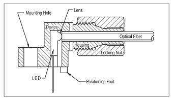
FIGURE 5. Cross-section of fiber optic device.
