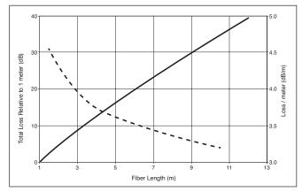
FIGURE 4. Fiber Loss in GH4001
