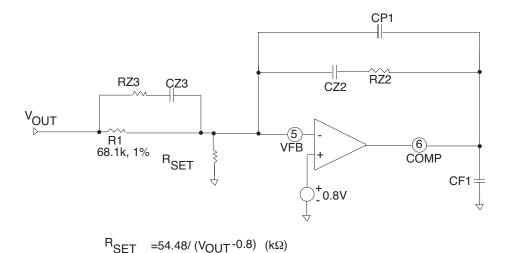
Type III Error Amplifier Compensation Circuit
