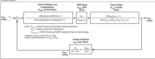
SP7650 Voltage Mode Control Loop with Loop Dynamic
