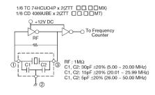
Figure 4) ZTT ... ... ... MX Test Circuit
