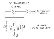
Figure 2) ZTT□.□□MG Test Circuit
