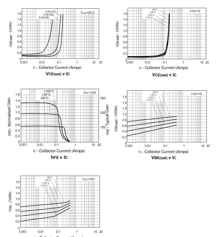
Ic - Collector Current (Amps) VBE(on) v IC
