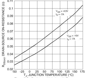
Figure 7 On-Resistance Variation with Temperature
