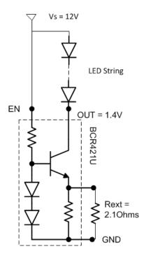
Figure 7 Example for 350mA operation
