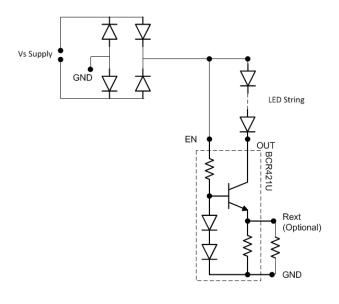
Figure 6 Application Circuit for LED Driver with Assured Operation Regardless of Polarity
