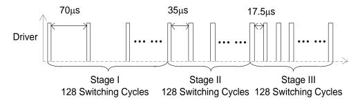
Figure 4. Driver Time Sequence in Startup Process
