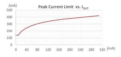
Figure 5. Frequency and Peak Current Limit Characteristic (Vo=12V, L1=1mH)
