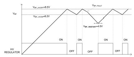
Figure 1.  $V_{\mbox{\footnotesize{BP}}}$  Waveform and HV Regulator ON/OFF Status
