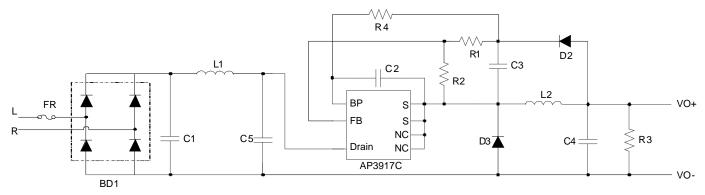
Figure 2. Low Standby Power Circuit with Auxiliary V<sub>BP</sub> Supply 6 of 12
