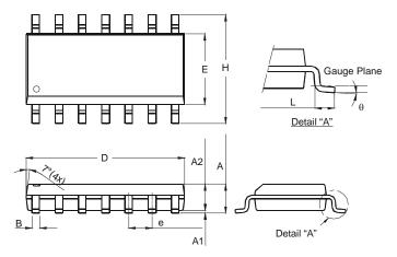
SO-14 Dim Min Max 1.47 1.73 А A1 0.10 0.25 A2 1.45 Typ В 0.33 0.51 D 8.53 8.74 Ε 3.80 3.99 1.27 Typ е Н 5.80 6.20 L 0.38 1.27 θ 0° 8° All Dimensions in mm
