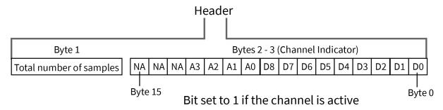
Sample data follows the header and the channel indicator frame determines how to read the sample data. If any of the DIO lines are enabled, the first two bytes are the DIO sample. The ADC data follows. ADC channel data is represented as an unsigned 10-bit value right-justified on a 16- bit boundary. The following figure illustrates the sample data bits.
