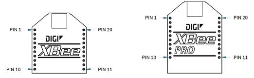
The following table shows the pin assignments for the through-hole device. In the table, low-asserted signals have a horizontal line above signal name.
