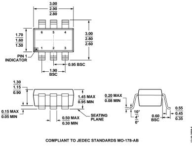
Figure 16. 6-Lead Small Outline Transistor Package [SOT-23] (RJ-6) Dimensions shown in millimeters
