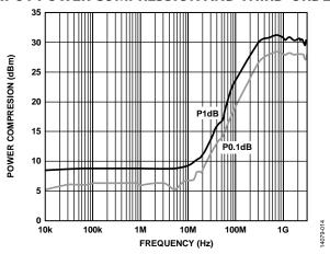
Figure 10. Input 1 dB Power Compression (P1dB) and Input 0.1dB Power Compression (P0.1dB) vs. Frequency,  $V_{CTL} = 0 \text{ V/5 V}$
