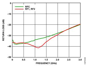
Figure 8. Return Loss vs. Frequency
