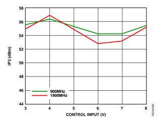
Figure 13. Input IP3 vs. Control Input Voltage
