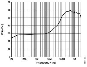
Figure 12. Input Third-Order Intercept (IP3) vs. Frequency,  $V_{CTL} = 0 V/5 V$
