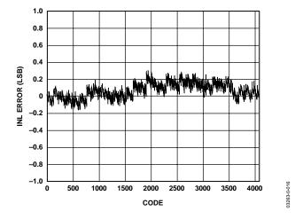
Figure 10. Typical INL,  $V_{DD} = 2.7$  V, Reference = 2.5 V, Mode1, 3.4 MHz f<sub>SCL</sub>, 121 kSPS
