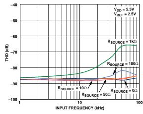
Figure 23. THD vs. Analog Input Frequency for Various Source Impedances for  $V_{DD}$  = 5.5 V, 136 kSPS, Mode 1
