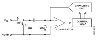
Figure 18. ADC Conversion Phase
