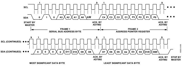
Figure 27. Two-Byte Write Sequence
