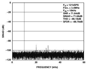
Figure 4. Dynamic Performance with 5 V Supply and 2.5 V Reference, 121 kSPS, Mode 1, Single-Channel Mode
