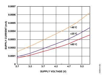
Figure 14. Shutdown Current vs. Supply Voltage, –40°C, +25°C, and +85°C
