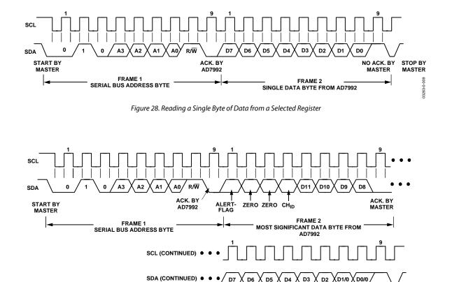
Figure 29. Reading Two Bytes of Data from the Conversion Result Register
