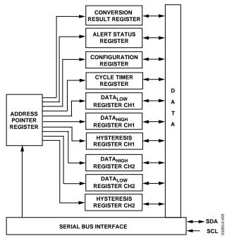
Figure 24. AD7992 Register Structure
