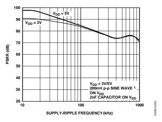
Figure 6. PSRR vs. Supply-Ripple Frequency, Single-Channel Mode Only
