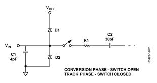
Figure 20. Equivalent Analog Input Circuit
