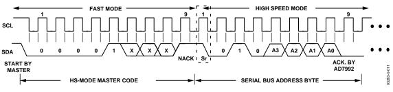
Figure 30. Placing the Part into High Speed Mode
