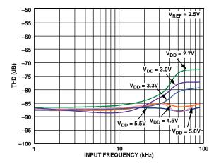
Figure 22. THD vs. Analog Input Frequency for Various Supply Voltages, Fs = 136 kSPS, Mode 1
