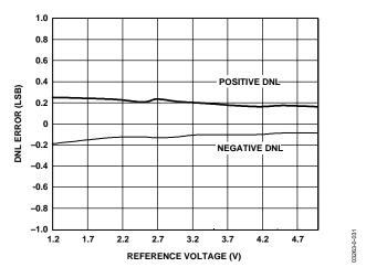
Figure 13. Change in DNL vs. Reference Voltage,  $V_{DD} = 5 V$ , Mode 1, 121 kSPS
