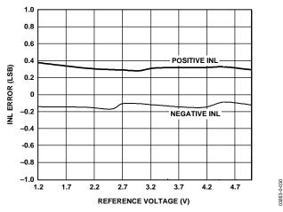
Figure 12. Change in INL vs. Reference Voltage, V<sub>DD</sub> = 5 V, Mode 1, 121 kSPS
