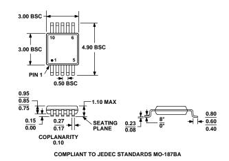
Figure 34. 10-Lead Mini Small Outline Package [MSOP] (RM-10) Dimensions shown in millimeters
