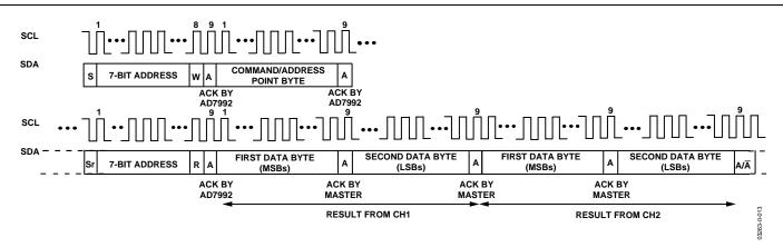
Figure 33. Mode 2 Sequence Operation
