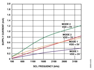
Figure 15. Average Supply Current vs.  $l^2$ C Bus Rate for  $V_{DD} = 3$  V and 5 V
