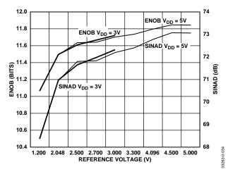
Figure 16. ENOB/SINAD vs. Reference Voltage, Mode 1, 121 kSPS
