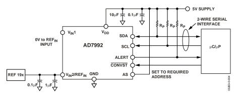
Figure 21. AD7992 Typical Connection Diagram, Single-Channel Mode, Mode 1
