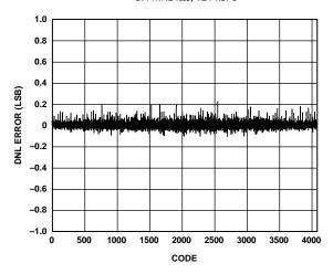
Figure 9. Typical DNL,  $V_{DD}$  = 5.5 V, Reference = 2.5 V Mode 1, 3.4 MHz f<sub>SCL</sub>, 121 kSPS
