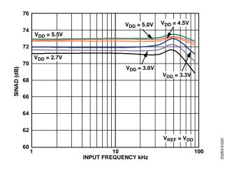
Figure 7. SINAD vs. Analog Input Frequency for Various Supply Voltages at 136 kSPS with 3.4 MHz f<sub>SCL</sub>
