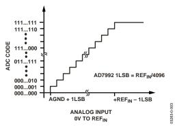
Figure 19. AD7992 Transfer Characteristic
