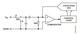
Figure 17. ADC Acquisition Phase
