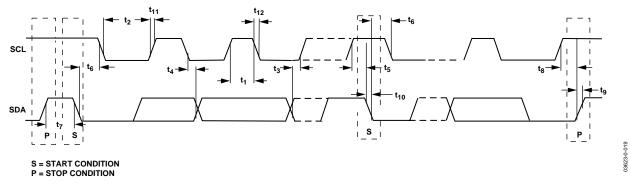
Figure 2. Two-Wire Serial Interface Timing Diagram
