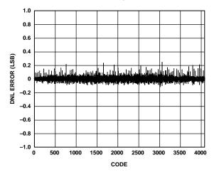
Figure 11. Typical DNL,  $V_{DD} = 2.7$  V, Reference = 2.5 V, Mode 1, 3.4 MHz f<sub>SCL</sub>, 121 kSPS
