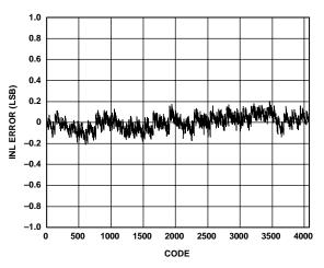
Figure 8. Typical INL,  $V_{DD}$  = 5.5 V, Reference = 2.5 V, Mode 1, 3.4 MHz f<sub>SCL</sub>, 121 kSPS
