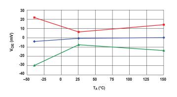
**Electrical Offset Voltage versus Ambient Temperature**
