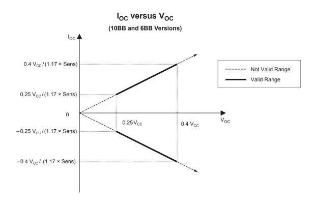
Example: For ACS709LLFTR-6BB-T, if required overcurrent fault switch point is 10 A, and  $V_{CC}$  = 3.3 V, then the required  $V_{OC}$  can be calculated as follows:
