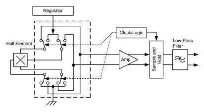
Concept of Chopper Stabilization Technique
