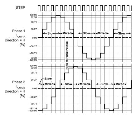
Figure 4. Decay Modes for Quarter-Step Increments
