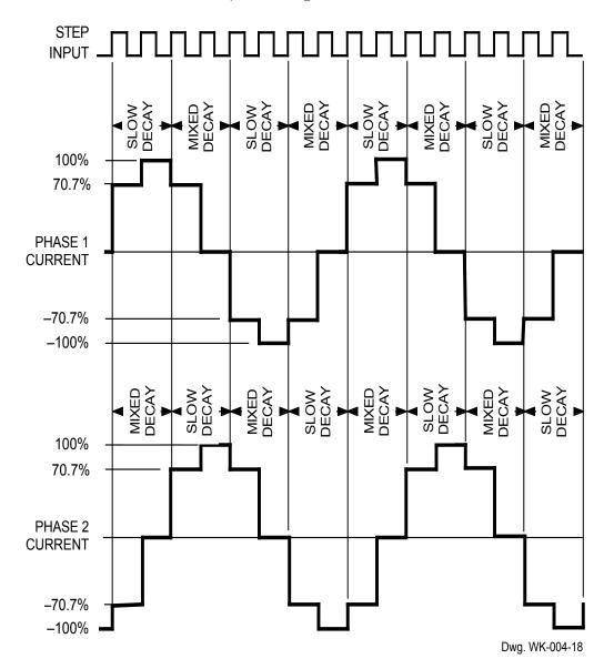
The mixed-decay mode is controlled by the percent fast decay voltage ( $V_{PFD}$ ). If the voltage at the PFD input is greater than  $0.6V_{CC}$  then slow-decay mode is selected. If the voltage on the PFD input is less than  $0.21V_{CC}$  then fast-decay mode is selected. Mixed decay is between these two levels.
