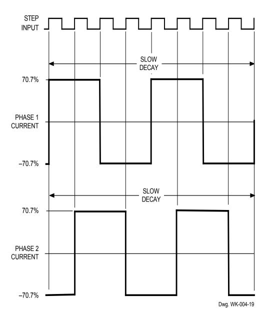
The vector addition of the output currents at any step is 100%.
