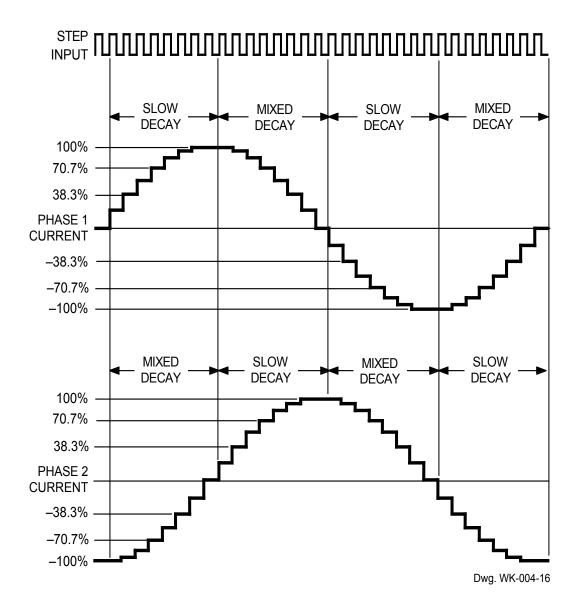
The mixed-decay mode is controlled by the percent fast decay voltage ( $V_{PFD}$ ). If the voltage at the PFD input is greater than  $0.6V_{CC}$  then slow-decay mode is selected. If the voltage on the PFD input is less than  $0.21V_{CC}$  then fast-decay mode is selected. Mixed decay is between these two levels.
