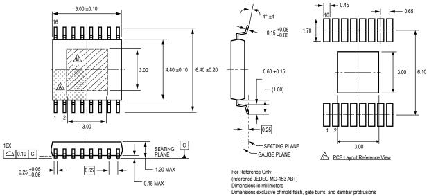
LP Package, 16 Pin TSSOP with Exposed Thermal Pad
