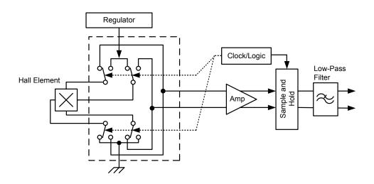
Figure 2. Model of chopper stabilization technique
