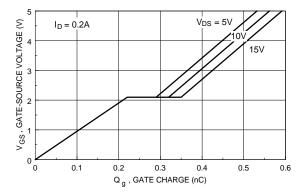
Figure 7. Gate Charge Characteristics.
