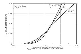
Figure 5. Transfer Characteristics.
