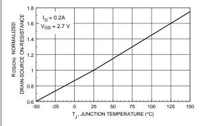
Figure 3. On-Resistance Variation with Temperature.
