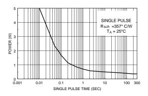
Figure 10. Single Pulse Maximum Power Dissipation.
