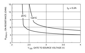
Figure 4. On Resistance Variation with Gate-To-Source Voltage.
