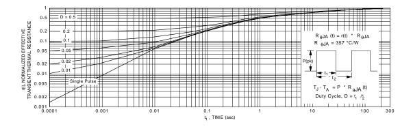
Figure 11. Transient Thermal Response Curve.
