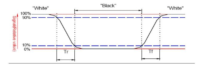
Note 6: Definition of contrast ratio: Contrast ratio is calculated by the following formula.
