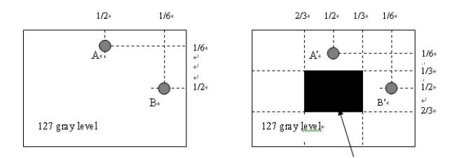
ILA-L A'I/LA X 100%= 2% max., LA and LA' are brightness at location A and A' ILB-LB'I/LB X 100%= 2% max., LB and LB' are brightness at location B and B'
