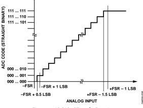
Figure 22. ADC Ideal Transfer Function
