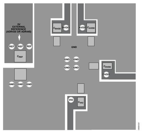
*Figure 39. Example Layout of the* AD7944 (Bottom Layer)
