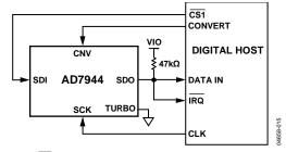
Figure 32. CS Mode, 4-Wire with Busy Indicator Connection Diagram
