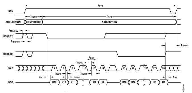
Figure 31. CS Mode, 4-Wire Without Busy Indicator Serial Interface Timing
