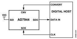
Figure 26. CS Mode, 3-Wire Without Busy Indicator Connection Diagram (SDI High)
