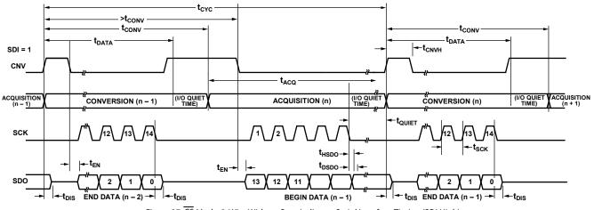
Figure 27. CS Mode, 3-Wire Without Busy Indicator Serial Interface Timing (SDI High)
