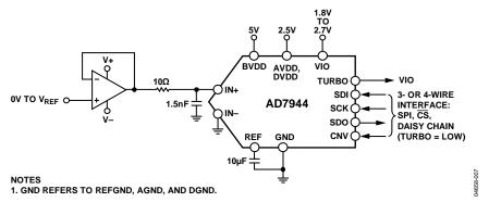
Figure 23. Typical Application Diagram with Multiple Supplies
