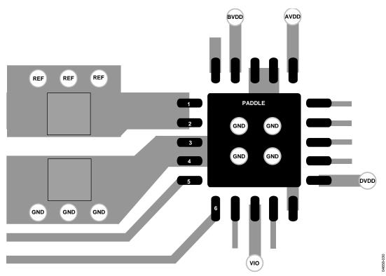
Figure 38. Example Layout of the AD7944 (Top Layer)
