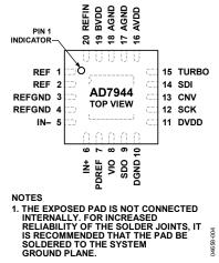
Figure 4. Pin Configuration
