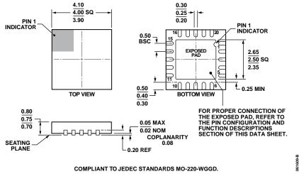
Figure 40. 20-Lead Lead Frame Chip Scale Package [LFCSP] 4 mm × 4 mm Body, and 0.75 mm Package Height (CP-20-10) Dimensions shown in millimeters
