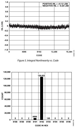
Figure 6. Histogram of DC Input at Code Center (External Reference)
