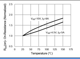
Fig.4 On-Resistance vs. Junction temperature
