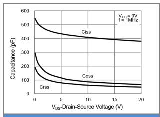
Fig.10 Capacitance vs. Drain-Source Voltage.
