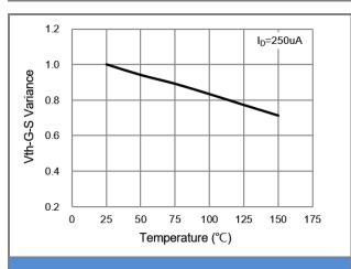
Fig.9 Threshold Voltage Variation with Temperature.
