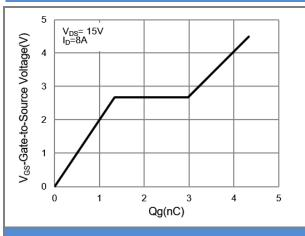
Fig.7 Gate-Charge Characteristics
