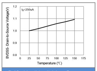
Fig.8 Breakdown Voltage Variation vs. Temperature
