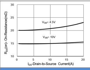
Fig.3 On-Resistance vs. Drain Current
