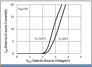
**Fig.2 Transfer Characteristics**
