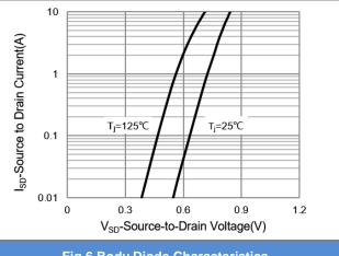
**Fig.6 Body Diode Characteristics**
